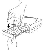
Place the disc onto the disc tray with the recording side of the disc facing the tray. Press down lightly until you hear the disc click into place. When placing the disc onto the tray, use your hand to hold the disc tray still.
