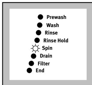
To select **Drain** only, press the “**Skip**” button three times, the **Wash - Rinse - Spin** LED,s go out.
