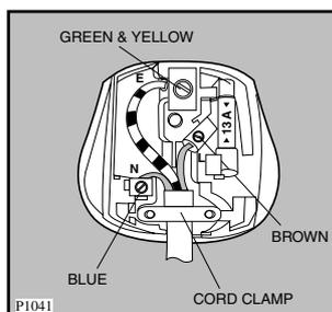
The wire coloured green and yellow must be connected to the terminal marked with the letter «E» or by the earth symbol  $\perp$  or coloured green and yellow.
