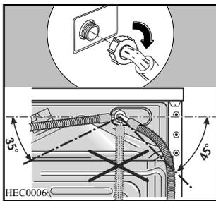
3. Set the hose correctly by loosening the ring nut. After positioning the inlet hose, be sure to tighten the ring nut again to prevent leaks.
